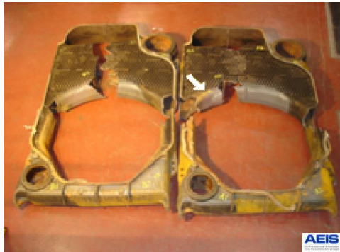
Figure 1: Assembly of broken segments of the Boiler Sections
