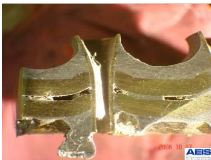
Figure 5: The void between the cover plate and the header plate
