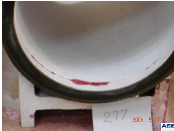
Figure 4: Crack in Cylinder liner 277
