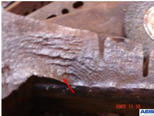
Figure 3: Origin of the main fracture as seen on the fracture surface
