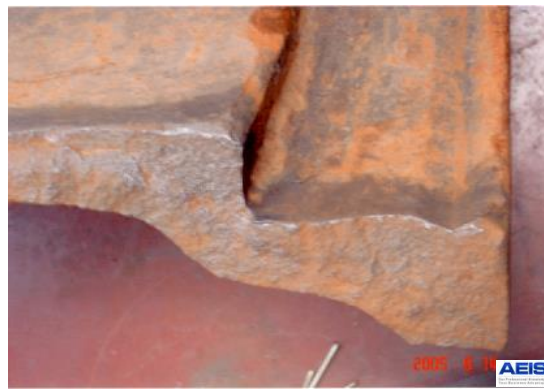
Figure 2: Cleaned fractured surface at Bell End
