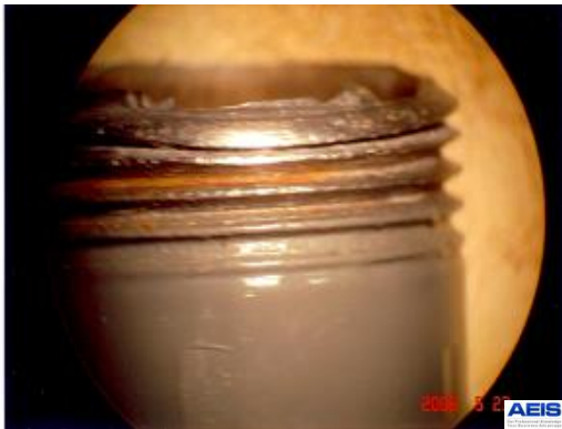
Figure 1: Metal deformation at the fractured end of the pipe
