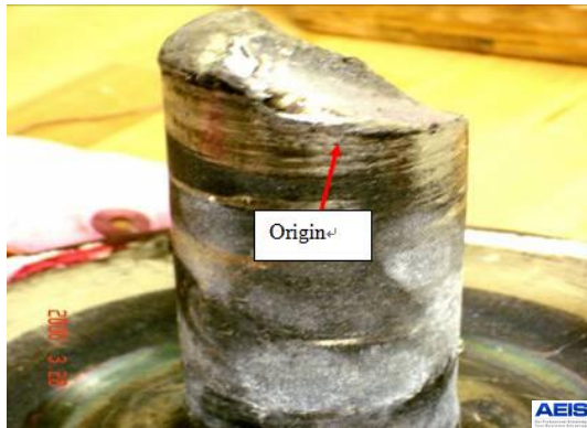
Figure 1: Scoring on the surface the flange end
