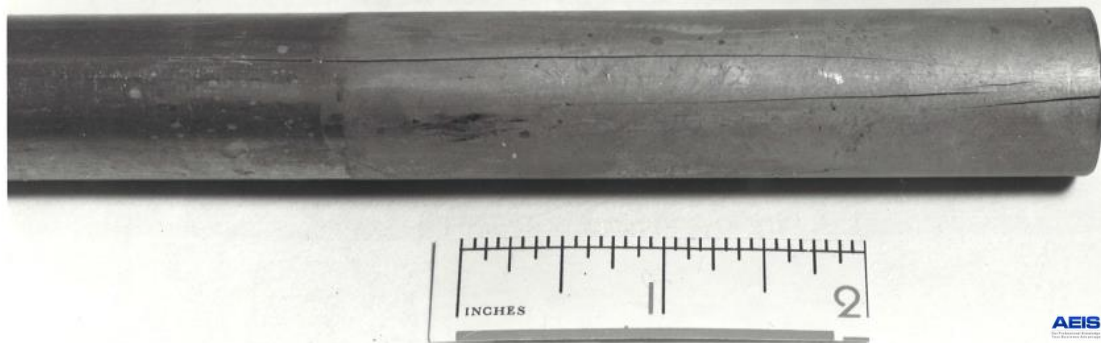
Fig 2 Cracking shows after mercurous nitrate test on NYCHA No.3
