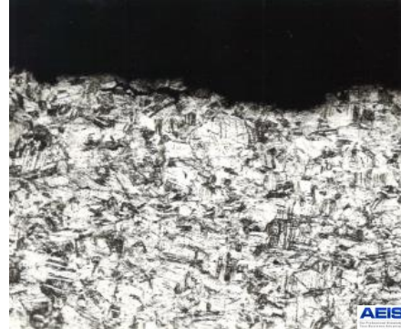
Fig 4 Intergranular cracking of No.1 pipe x200
