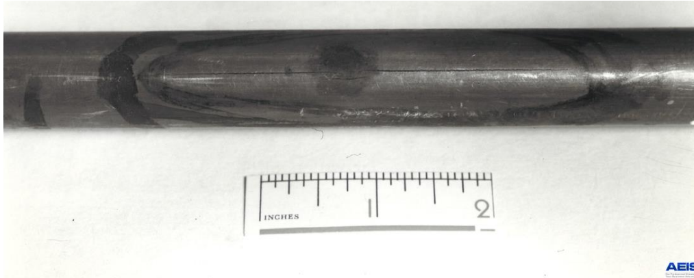
Fig 1 Crack on “NYCHA NO.1”
