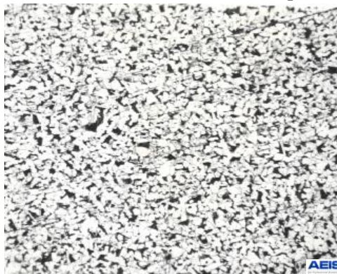
Fig 5 Microstructure of the fractured drive shaft X100
