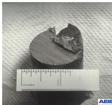
Fig 3 Fracture site at the end of keyway
