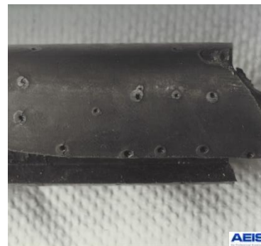
Fig 4 Fracture begun through one of the punch marks
