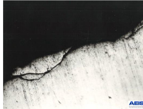
Fig 2 Cross-section of fractured surface X500
