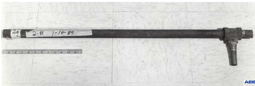
Fig 1 Pipe with pinhole at the end as received condition
