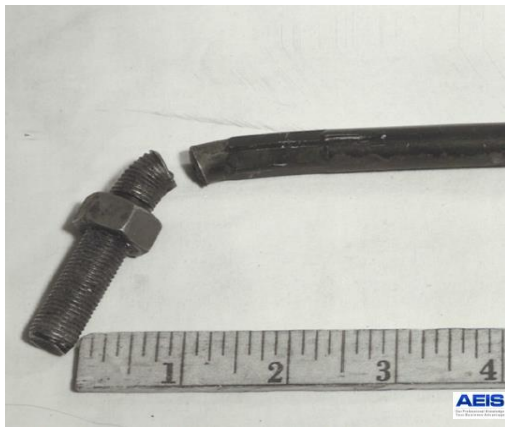
Fig 1 Fracture tie rod as received condition
