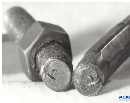
Fig 2 Close look of fracture surface
