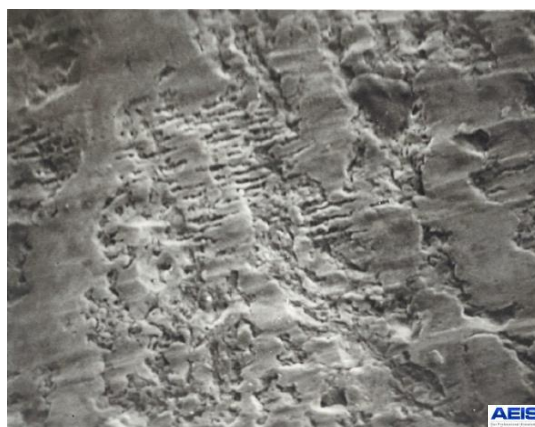
Fig 3 SEM of “MIDWEST” disc shows typical fatigue structure X600
