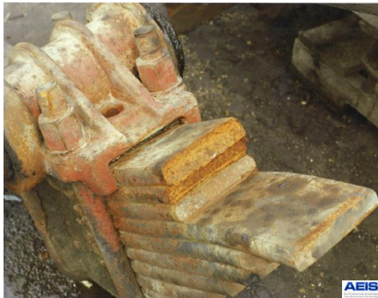
Fig 1 Fractured Leaf Spring as received condition
