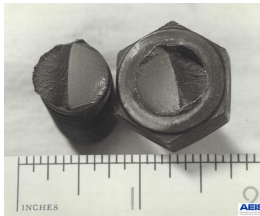
Fig 1 Fractured cap screw as received condition showing a fatigue fracture structure
